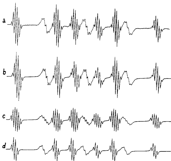
Figure 4. Experimental spectrum of the PSt nitroxide chiral radical pair at 80 °C (a) and its simulated version (b). The theoretical spectrum (b) consists of two components (c and d) which are superposed with equal weights. The best fitting spectrum parameters are as follows: (c) g = 2.0066 , a_N = 1.290 mT, a_{H_\beta} = 0.925 mT, a_{H_{m,p}} = 0.058 mT, a_{H_\gamma} = 0.120 mT; (d) g = 2.0066 , a_N = 1.300 mT, a_{H_\beta} = 0.915 mT, a_{H_{m,p}} = 0.060 mT, a_{H_\gamma} = 0.005 mT.
